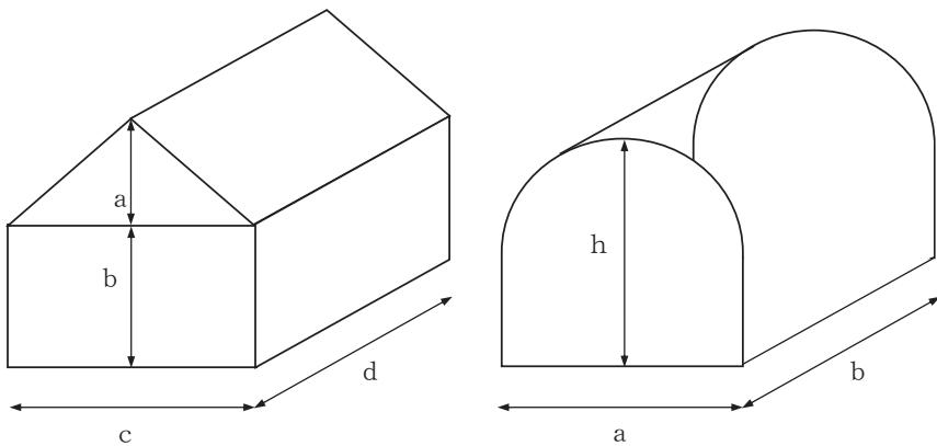
$$\text{容積} \doteq 80/100 \times (a+b) \times c \times d$$
